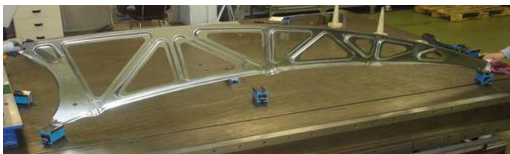
Figure 28 Stamped cantilever arm by Sener; the design was developed to reduce material and energy demand
